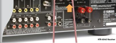
Connect Surround Speakers Positive (+) side of the wire with white stripe attaches to (+) terminal. Negative (-) side attaches to (-) terminal.
